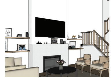
Fireplace Details Plaster Surround with Painted Drywall Above
